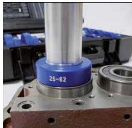
Collets are engraved and marked clearly
